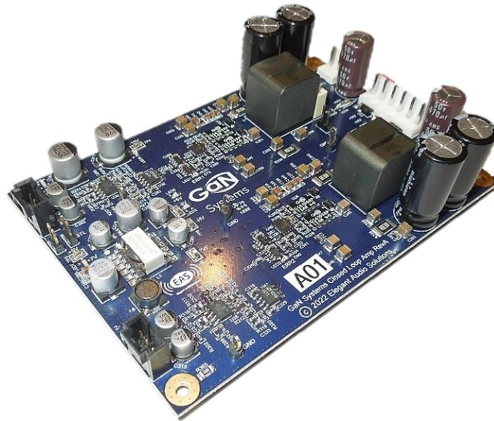
Figure 1 GS-EVM-AUD-AMPCL1-GS Evaluation Module
