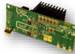
Half bridge power stage
