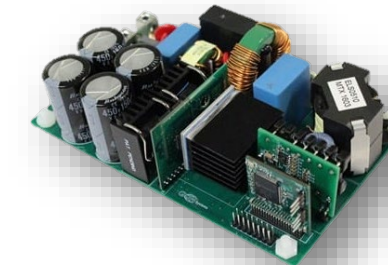
1.5 kW bridgeless totem pole PFC
