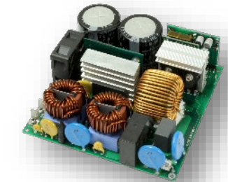
3 kW bridgeless totem pole PFC
