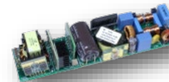
1.5 kW bridgeless totem pole PFC
