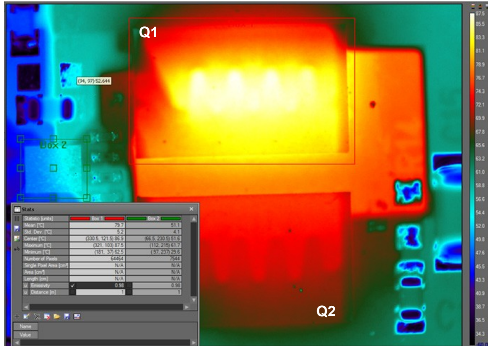
Figure 11 • GS61008P-EVBHF Evaluation Board with Fan On ( T_{MAX} = 87.5^{\circ}\text{C} )
