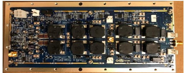
Fig.10. 150W Air Fuel high power PA close up view
