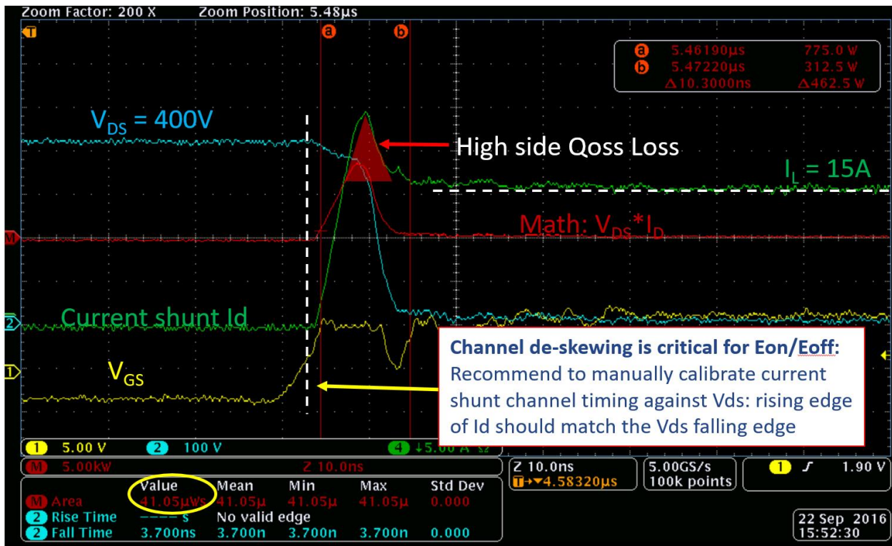
Figure 19 Turn-on switching loss measurement ( E_{on}=41\mu J , 400V/15A)
