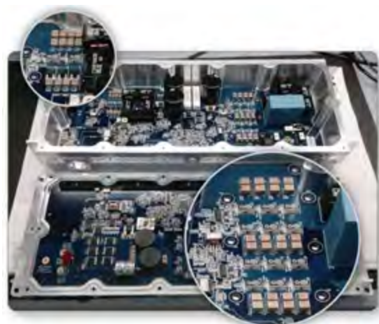
Figure 3: 2kVI Vehicle Inverter Using GaN Switches in a Full-Bridge Configuration
