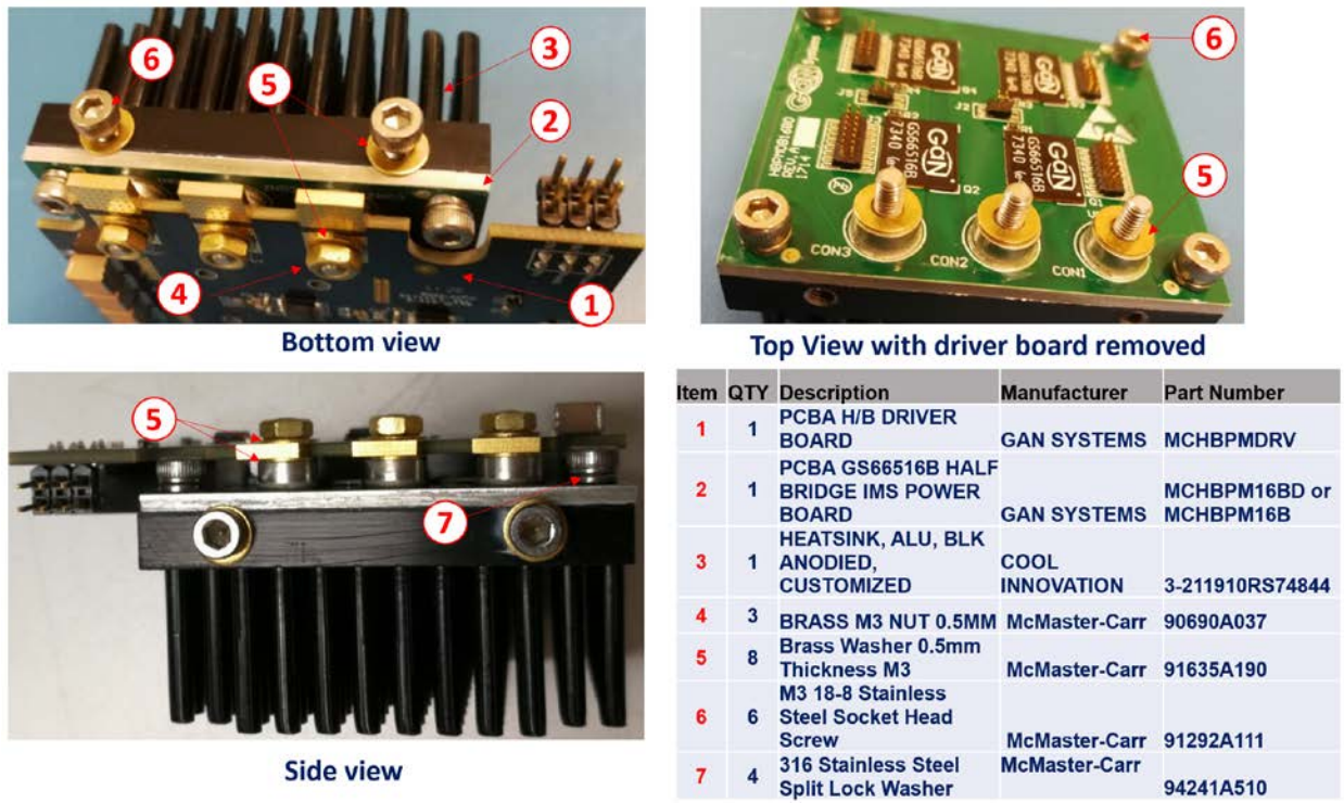
Figure 10 - IMS evaluation module assembly
