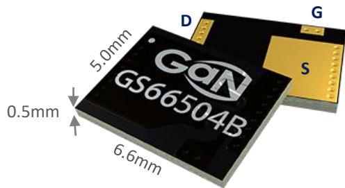
GS66504B/GS66502B (650V, 15/7A, 100/200mΩ)
