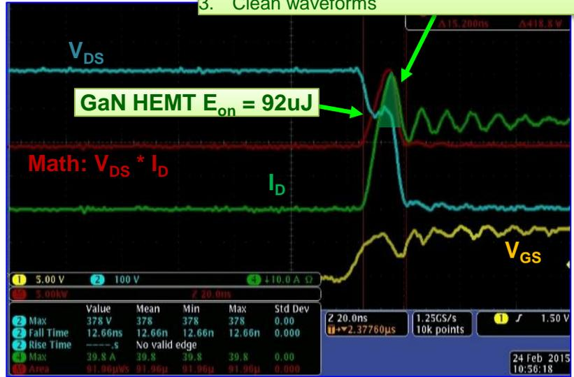
Hard switching turn-on of a GaN E-HEMT @ 400V/22A
