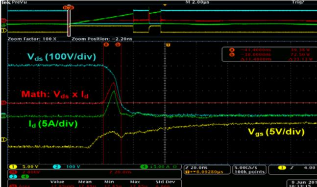
400 V<sub>dc</sub> with T<sub>j</sub>=75°C and R<sub>g\_on</sub>=30 ohm
