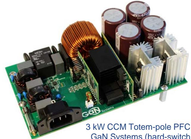
3 kW CCM Totem-pole PFC from GaN Systems (hard-switching)
