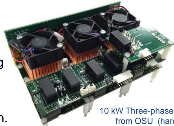
10 kW Three-phase traction inverter from OSU (hard-switching)
