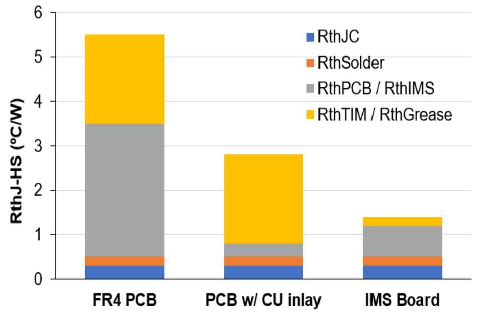
**The thermal performance is enhanced compared with the PCB solution.**
