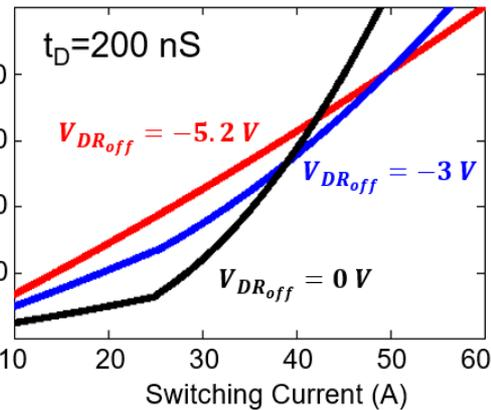
Half-bridge overall loss vs. switching current under different negative turn-off gate voltage  $V_{DRoff}$  (a) with deadtime  $t_D=40 \text{ ns}$ , (b) with deadtime  $t_D=100 \text{ ns}$ , (c) with deadtime  $t_D=200 \text{ ns}$ .
