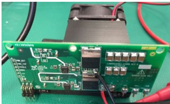
Figure 11: C3M0065090J Thermal Resistance Setup
