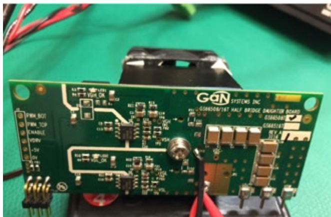
Figure 10: GS66508T Thermal Resistance Setup
